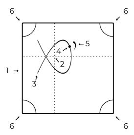
The centre point (2) as well as the rotation and size of the Orbiter trajectory can be set from the touchscreen interface. When **Retrigger** → is enabled, the Orbiter motion always starts from the beginning of the shape – its zero phase (3) – on note input or after each cycle of the Arpeggiator sequence. Note that the zero phase can be changed by Warp.
