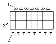
The arpeggiator note memory can be temporary (with arpeggiator playing only the currently pressed notes), **Latched** (notes stay in memory even after they are released), or **Steprecorded** • REC. The order in which the notes are played out can be sorted **Up** •, **Down** • or **Shuffled** .
