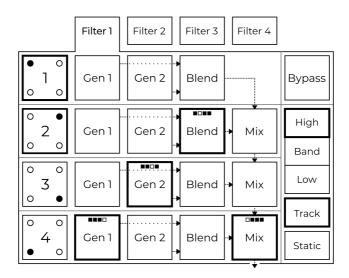
The picture above shows the Corner Matrix interface with four tabs representing each filter and four rows corresponding to each Corner.
