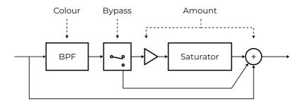
The **Bypass**: button on the **Effects screen** †† disables the saturator. In this case, the **Drive Amout** only sets the mix level of the effect's band-pass filter.
