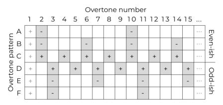
Patterns A–C include even-*ish* overtones while patterns D–F are more odd-*ish* (note that the 1st overtone, the fundamental, is always present). Some overtones are present with positive and other with negative amplitudes, making it possible to subtract overtones when blending two patterns together.
