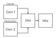
In the **Combined PM+AM modulation** mode, Generator 2 frequency-modulates Generator 1, and then the result is audiorate amplitude cross-modulated between the frequencymodulated Generator 1 and the original Generator 2.
