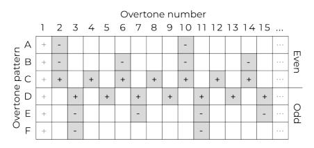
Patterns A–C include even overtones while patterns D–F include odd overtones (note that the 1st overtone, the fundamental, is always implied unless turned off in the Prime Slot tab of the Corner Matrix). Some overtones are present with positive and other with negative amplitudes, making it possible to subtract overtones when blending two patterns together.
