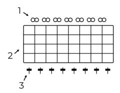
The chaining either generates legato in the Mono polyphony mode or joins two steps with equal octaves in the Dual and Poly modes.
